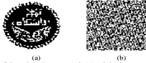
Fig. 4. The Arnold transform of the original watermark (a) original watermark (b) transformed watermark
